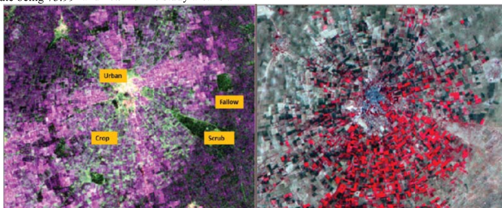
Figure 1: (a) FCC of L-band PALSAR image (b) LISS-III FCC corresponding to (a)
