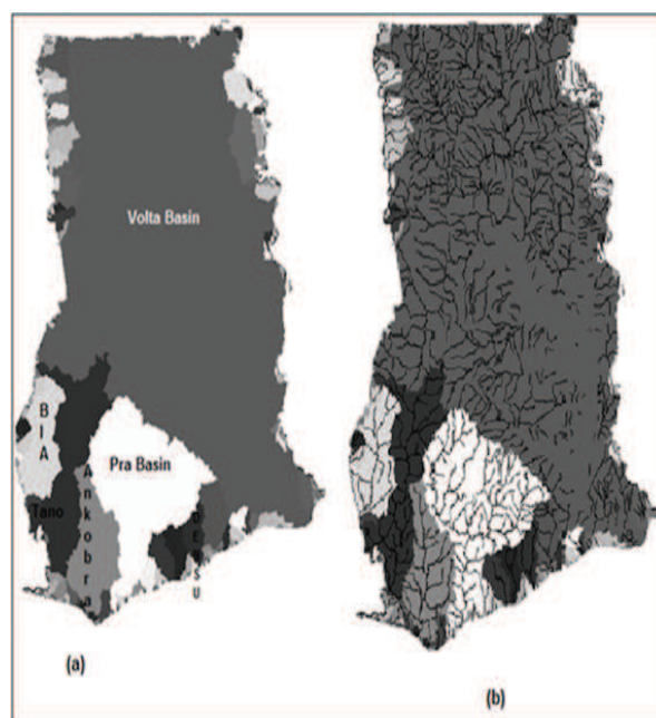
Figure 3: (a) The estimated watersheds boundaries of Ghana and (b) overlay of a digitized river network (Mårtensson et al., 1999) on the estimated watersheds.
