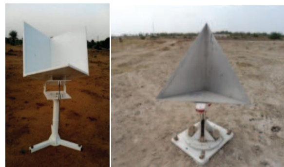
Figure 6: Trihedral corner reflectors used for calibration analysis (a) Square trihedral of size 75cm (b) Triangular trihedral of size 90cm. (source: NRSC (Hyderabad); SAC(Ahmedabad))
