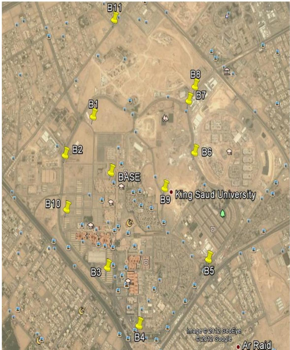
**Figure 3: The distribution of the GCPs (Ground Control Points) in the study area**
