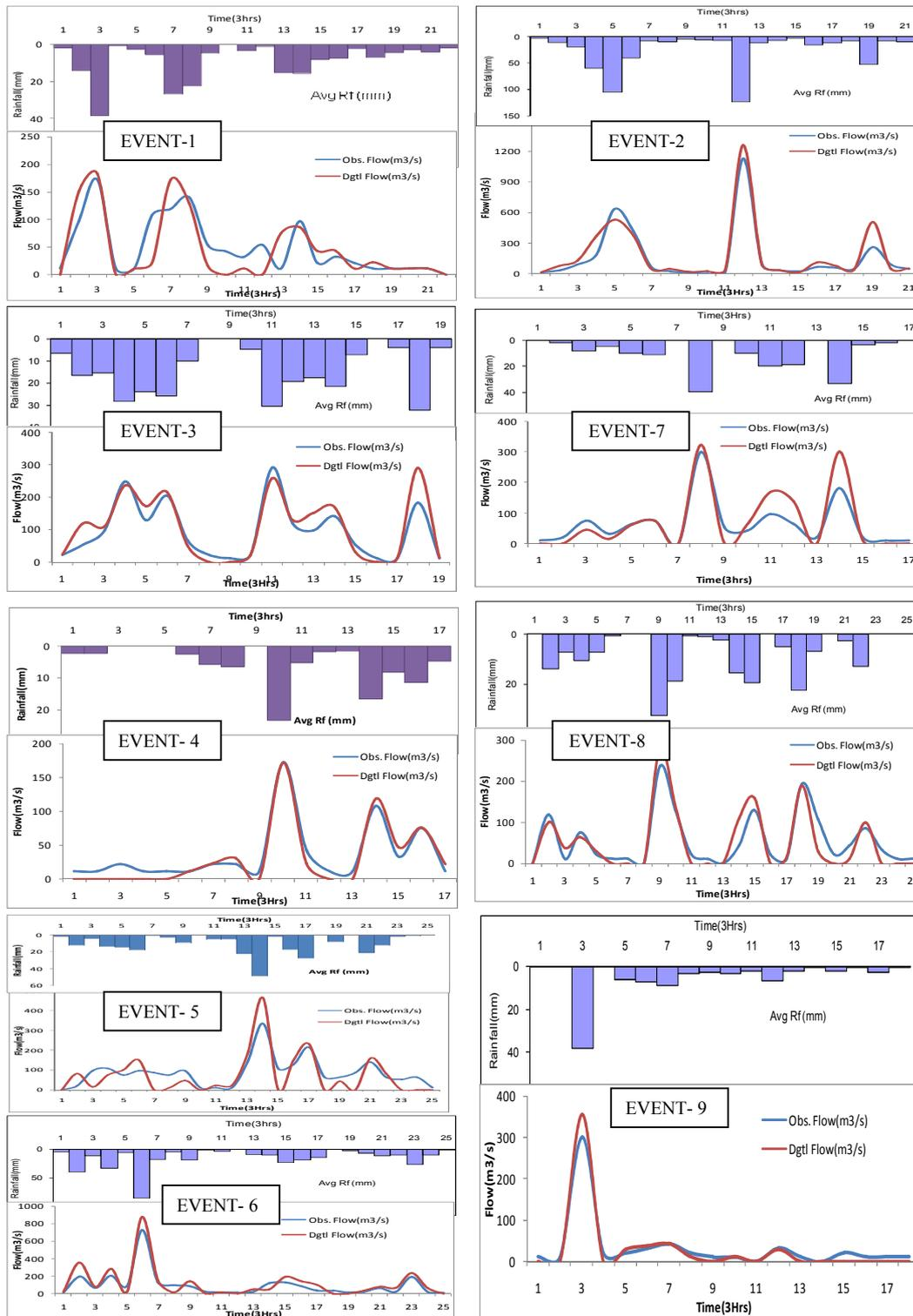
Fig. 7: Digital runoff results with observed Hydrographs
