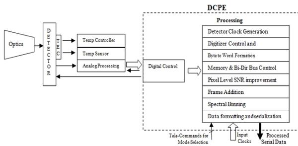
**Figure 1: The diagram of Thermal infra-red (IR) Imaging Spectrometer (TIS)**
