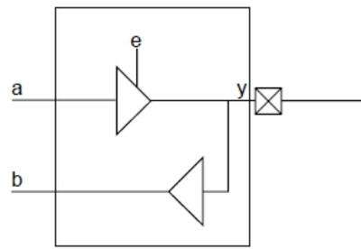
**Figure 4: Bi-directional buffer in FPGA library**
