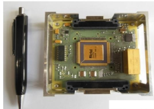
**Figure 5: DCPE card in assembled package**
