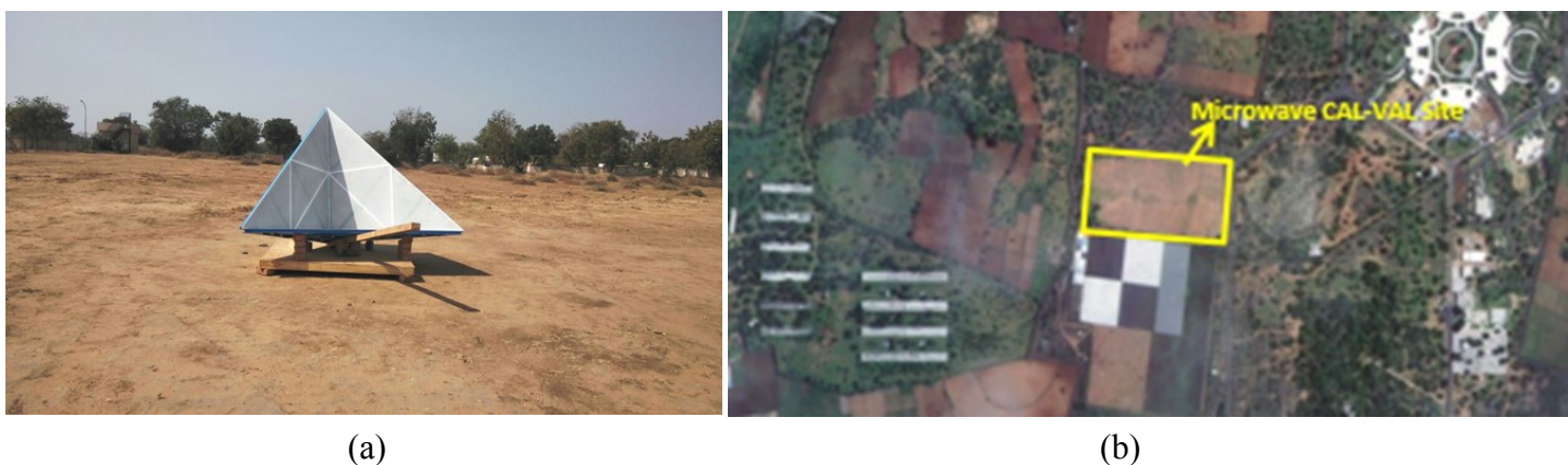
Figure 6: (a) Field snap of one of the deployed 2m perforated CR at SAC-Bopal site (b) Location of permanent Indian CR network at NRSC-Shadnagar on Bhuvan
