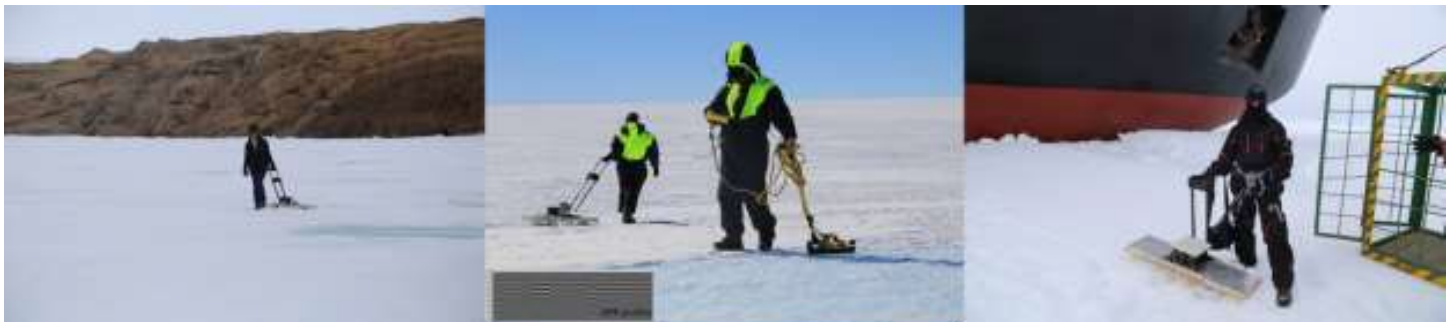
Figure 7: GPR survey on fast ice and sheet ice
