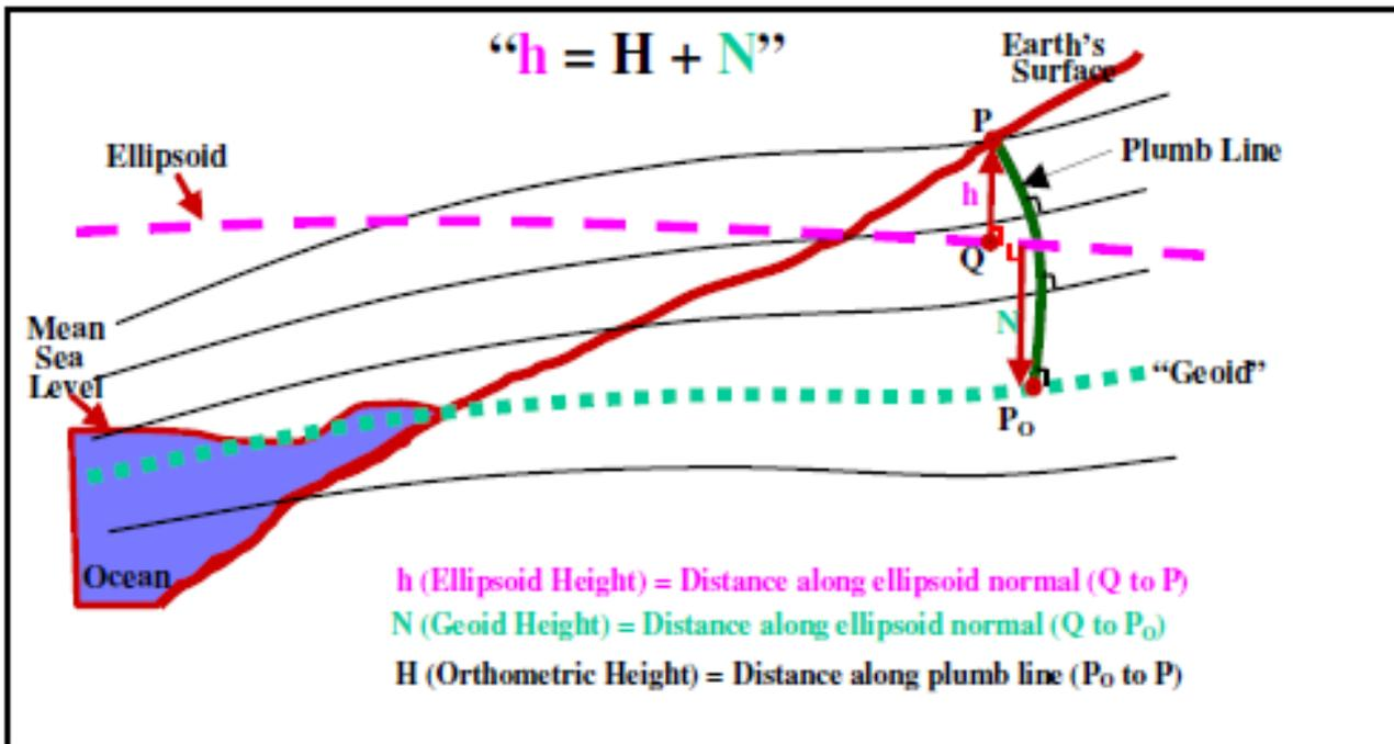
Figure 1: Relationship between geoid, ellipsoid and orthometric heights (Source: Roman et al., 2010)
