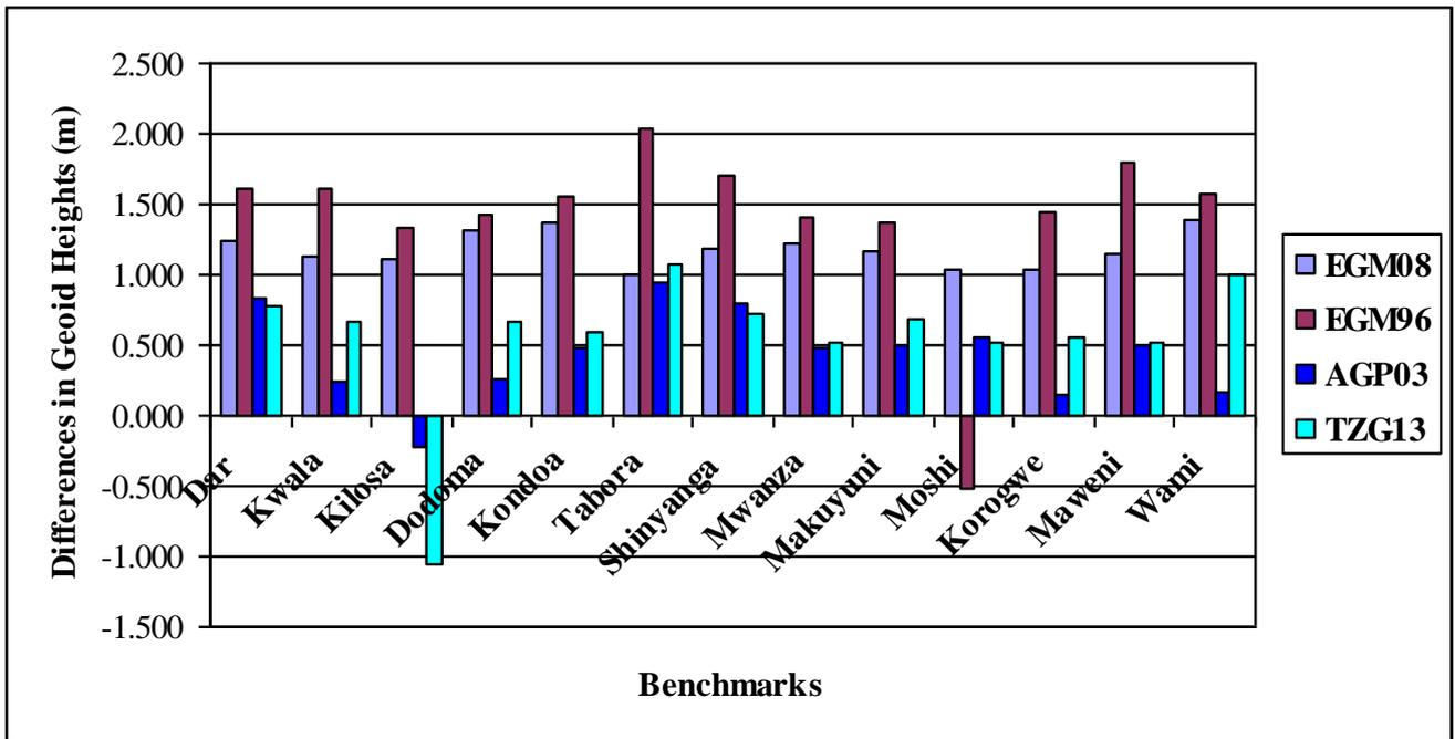
Figure 4: Comparisons of absolute differences of the predicted geoid heights from each model based on GPS/levelling derived geoid heights
