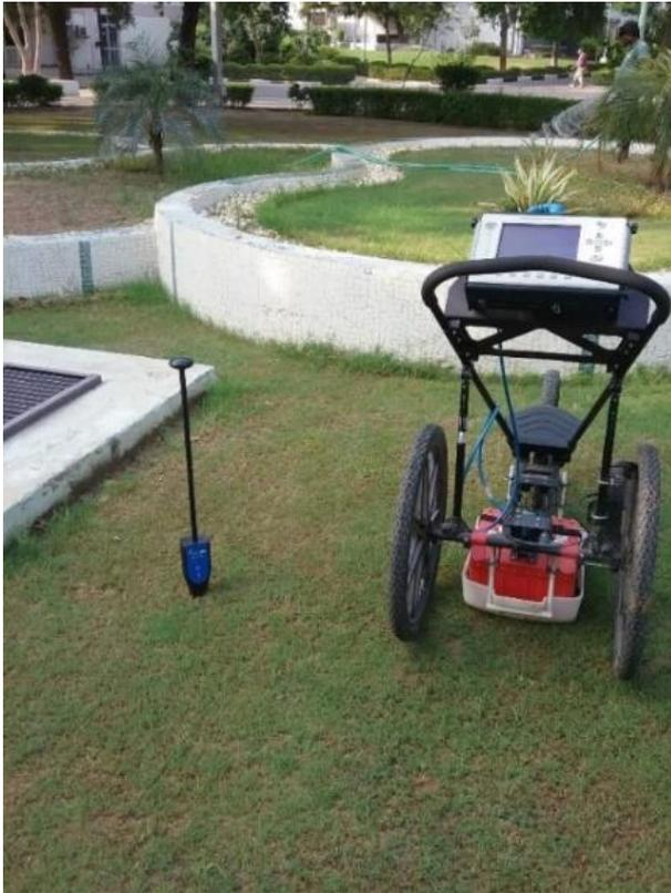
**Figure 4: GSSI 400 MHz GPR antenna (red) with control panel and carrier three-wheel cart. Left side HydraGo (blue) soil moisture instrument for measuring dielectric constant of soil.**
