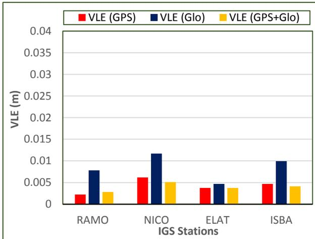
**Figure 4: Vector Length Errors (VLE) for different baseline lengths by using the three solutions (12 hrs) in 2014**
