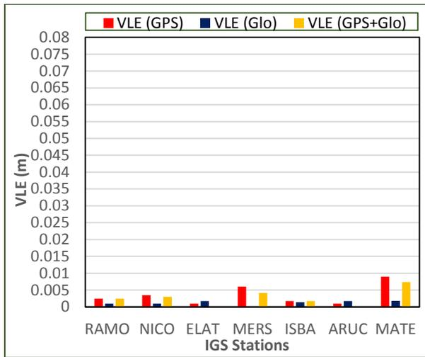
**Figure 11: Vector Length Errors (VLE) for different baseline lengths by using the three solutions (20 hrs) in 2018**
