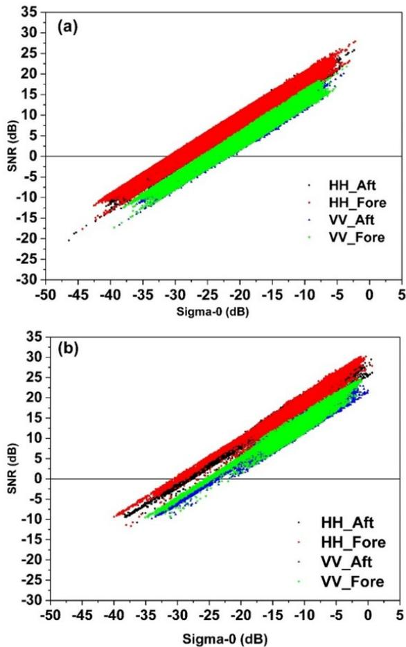
**Figure 9: Sigma-0 vs SNR for inner and outer beam over (a) sea (b) land**
