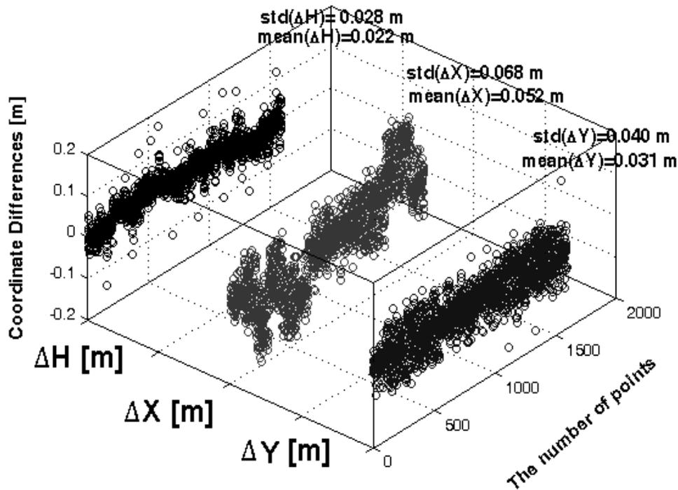
Figure 9: Comparison of the obtained coordinates of the points by using VRS-FKP in three days
