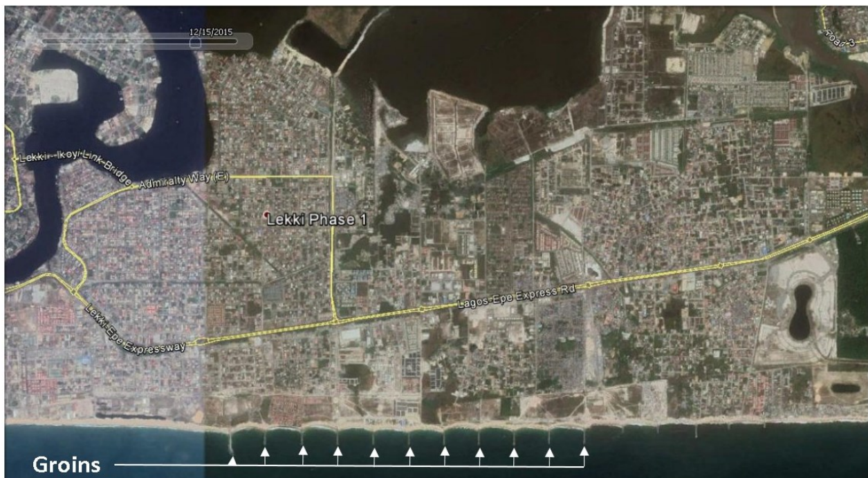
Figure 9: Newly constructed groins off the Lagos coast (Imagery source: Google Earth, December 2015)
