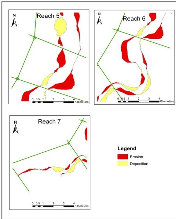
**Figure 3: Erosion/deposition (Reach 5 to Reach 7) in various reaches of Manas-Beki River over a period of 7 years (2008-2015)**
