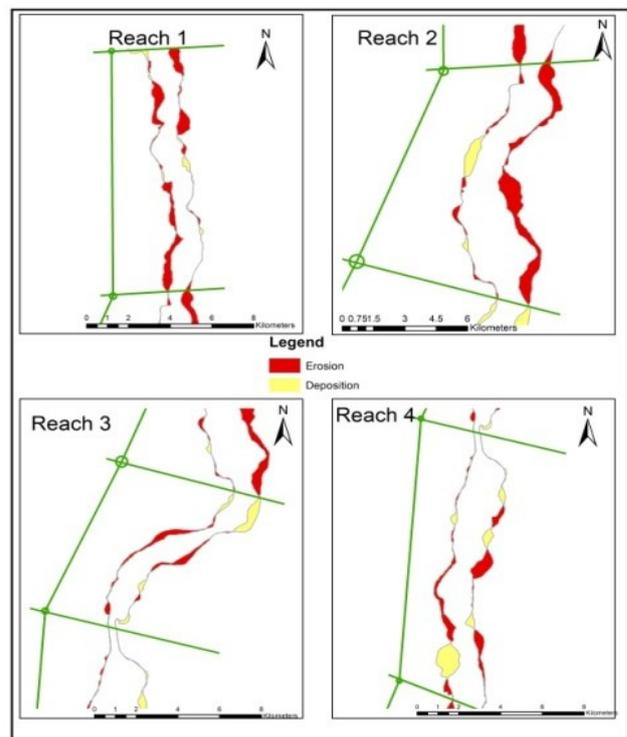
Figure 2: Erosion/deposition (Reach 1 to Reach 4) in various reaches of Manas-Beki River over a period of 7 years (2008-2015)
