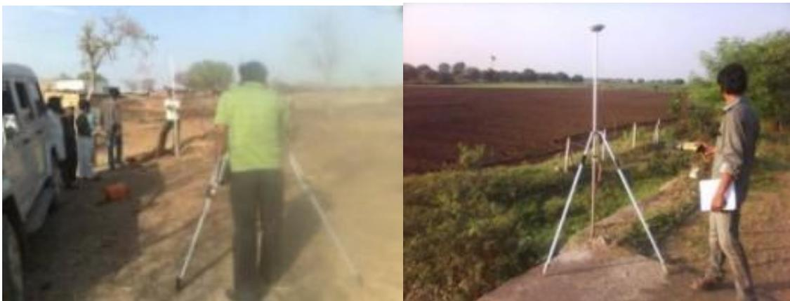
Photo 1. Field Survey of DGPS and Double Fly Levelling
